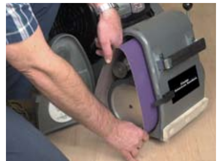
Recessed drum door provides better air seal and eases abrasive installation and adjustments
