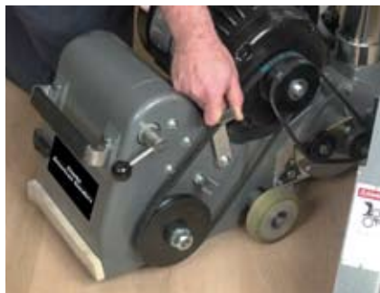
Quick release drive belt tension system eases disassembly and storage
